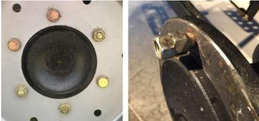
G. You will need to remove the 2 Stud on the axle, double nut tight the Stud as in photo & turn counter clockwise the inside nut. The stud should unscrew itself from the axle.
