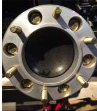
H. Get your Tire/Rim & add Loctite to the 6 studs on the spacer. You will need to use the supplied nuts that came install on the Spacer (M16x1.5) & use the supplied lock washer to install the rim/wheel. Torque the nuts to 140 ft. lbs for the rear wheels in the same 3 steps as above.
